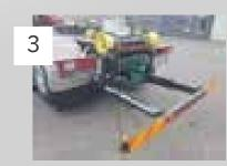
PANTO rear underrun protection adjustable or fixed
